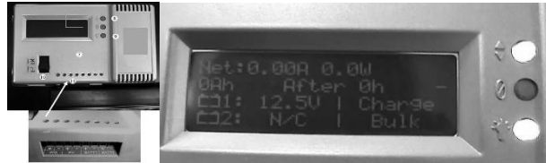
Fig. 3 The liquid crystal display of the charge controller is integrated with the front panel control console, which includes its connection terminal.
