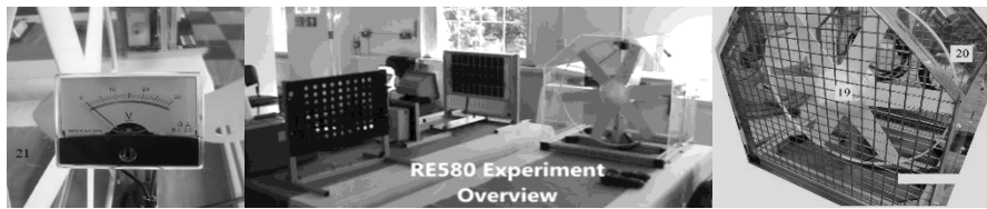
Fig. 1 Overview of the Combined Wind Turbine - Photovoltaic Panel Test Bench The Mini Wind Turbine with its Transparent Protective Housing and Built-in Voltmeter
